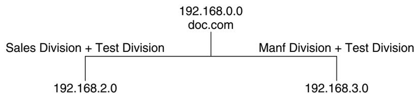
Traffic for the Test Division would not have its own subnet, but would instead be split between 192.168.2.0 and 192.168.3.0. However, with a network information service, the Test Division traffic could have its own dedicated network.
