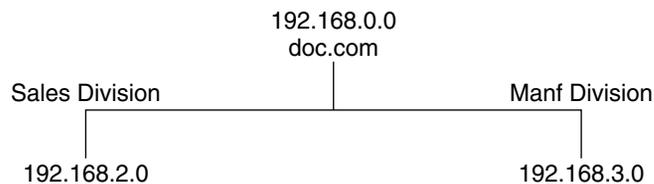
Each division could be identified by its network address, as shown above, but descriptive names made possible by naming services would be preferable.
